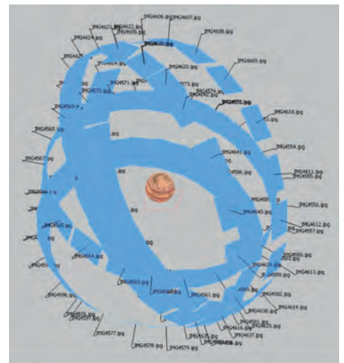
The image above shows the photos taken to create the 3-D model of the lid: a total of 64, taken from different perspectives. Below, the same image for the body of the vessel, for which a total of 92 photos were taken.
