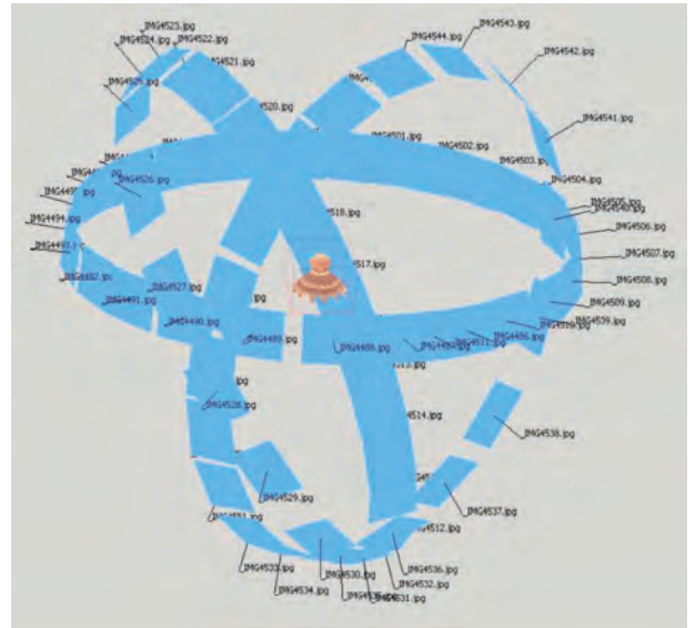
The image above shows the photos taken to create the 3-D model of the lid: a total of 64, taken from different perspectives. Below, the same image for the body of the vessel, for which a total of 92 photos were taken.
